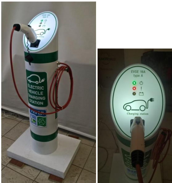
Fig. 6: The EVs charging station that will be fed by the second microgrid.
