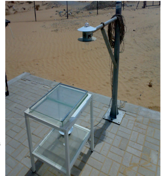
Comparison of Solar Transmittance of PCM with Water and Air.
