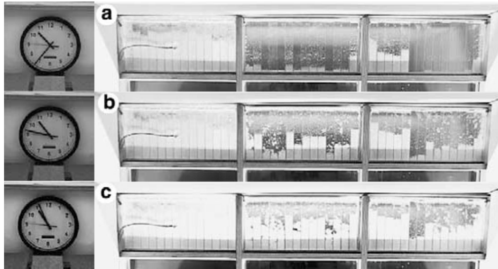
Freezing process of a Paraffin Wax
