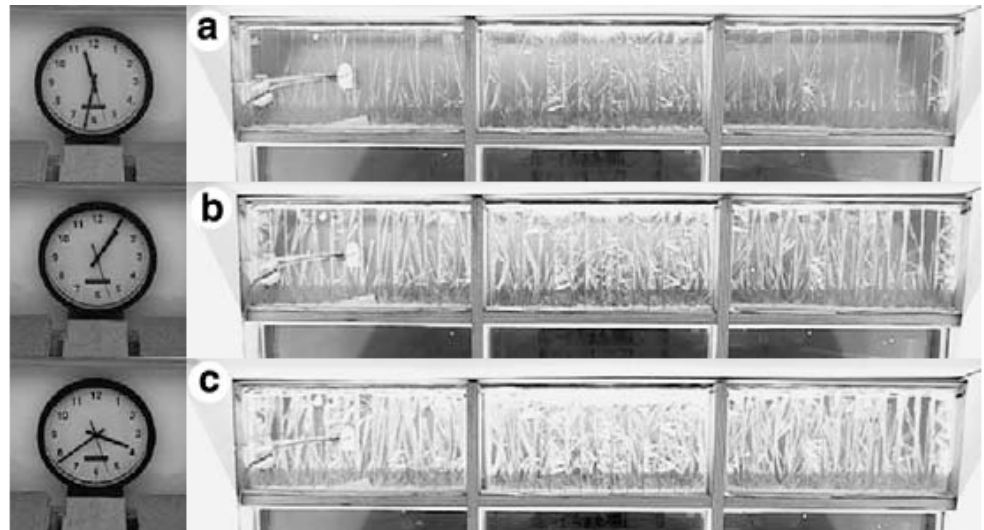
Freezing process of a Salt Hydrate
